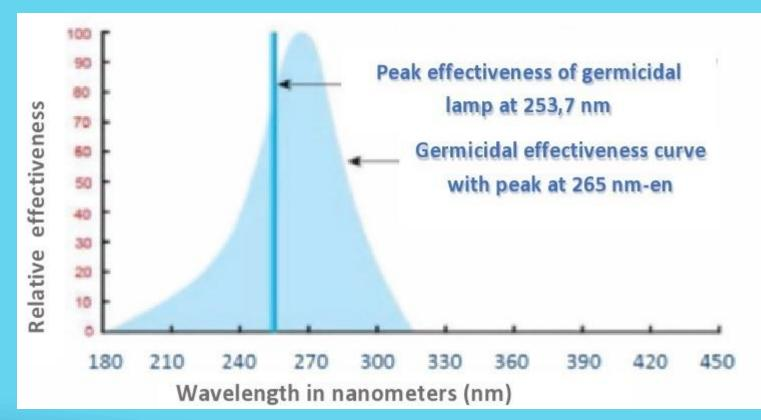
The low pressure R-FILTER germicidal lamps have the most effective action at 253,7 nm. This is close to the peak of the germicidal effectiveness curve.
