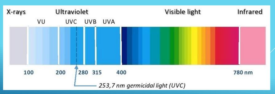
At the wavelength of 265 nm, the germicidal effect of UV-C radiation has its maximum.
